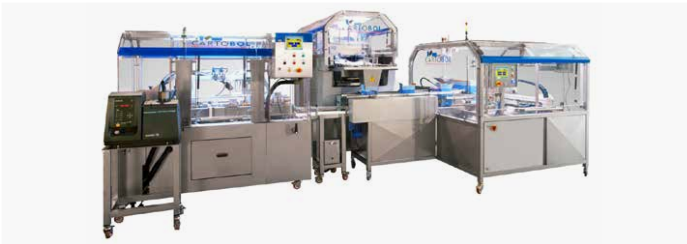
Fully Automatic Bag In Box Line – Case Erector – Filler – Inserter And Case Sealer
