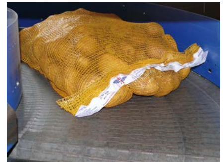
The allowed belt load of the Puma is 1850 kg/meter belt width, ideal for heavy loads such as potato bags.
