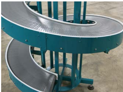
The JP Puma Spiral is a vertical conveyor for handling large numbers of unit goods such as bags, boxes and cartons.
