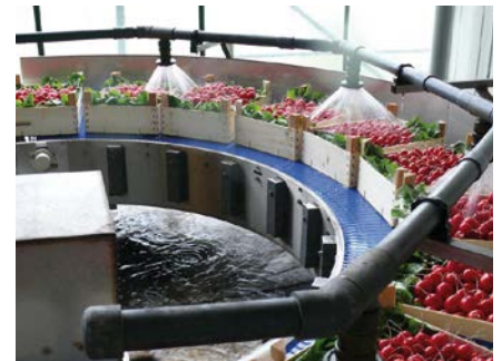
The blue belt of the Puma Compact Light is made of food-approved Poly Amid (FDA and EU10/2011).
