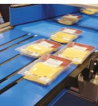
The Packleader BCS range of high speed convergers is designed to take multi-lane production of thermoformed packs and converge them at accurate spacing into a single lane.
