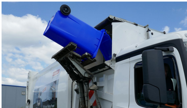
Lifting and emptying test
