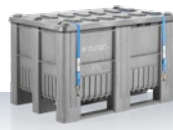
CB1 | 470 L 4H2/Y438/S/.../D/BAM 15814-CR ① 1200 x 800 x 740 mm ② 1236 x 836 x 765 mm Max. gross weight: 437,5 kg Standard colours: ■
