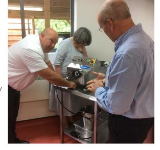
a semi-automatic volumetric benchtop unit, the Response efficiently fills a wide range of product viscosities, including LittlePod's extracts and pastes, with equal ease. The Response is quick to assemble and clean, meaning that changing between products and containers is as easy as possible and production downtime is kept to a minimum; LittlePod can swiftly switch from filling paste into 100ml aluminium tubes, to extracts in 100ml glass bottles, as required.
